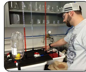
Device to Teach Hydraulic Analogy
