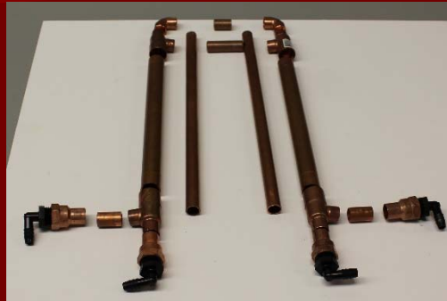
Disassembled view of double pipe heat exchanger
