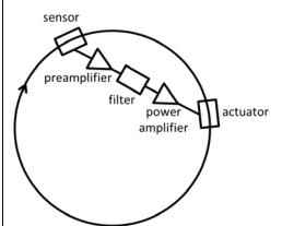
**Figure 1.** The introduction of a filter into the feedback control system for stochastic cooling, adapted from Fig. 7 of [2].
